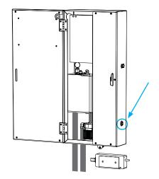
Fill the reservoir with distilled water until the reservoir is full. It is normal for the pump to start and stop a few times during filling. A water level sensor inside the tank ensures that the pump stops when there is water missing.
