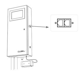
Be sure to always test your wire with an RJ45 wire tester before plugging the wire into the device. Reversing two wires when installing the connector could damage the product electronics.
