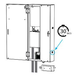
6 Repeat step 5 a minimum of three times to make sure the system is full of water.
