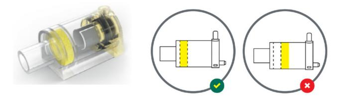
Replace the entire sensor assembly every two years. Disconnect the connector and tube from the water filter by pulling them off. Remove the sensor from the condensation pan. If water is present, place a bucket underneath to catch it. Install the new sensor and reconnect everything.
