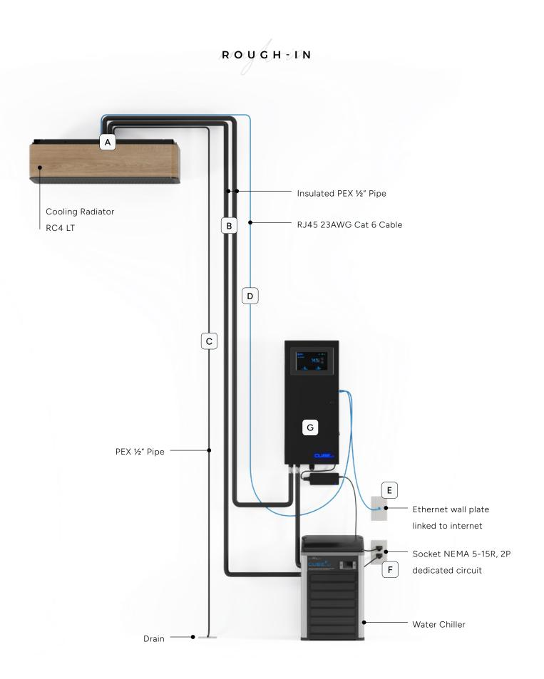
Position RC4LT in the wine cellar. It is important to consider the thickness of the insulation, finishing material and glass envelope when locating the final location of the unit.
