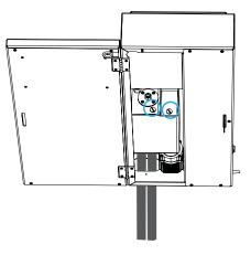
5 Close the door and lock the front of the control box using a coin.
