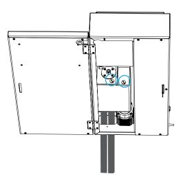
3 Fill the tank with distilled water until the tank is full. It is normal for the pump to start and stop a few times during filling. A water level sensor inside the tank ensures that the pump stops in the event of a lack of water.
