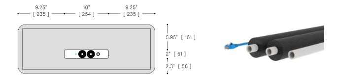
B Install 2 x 1/2" insulated PEX pipes between the location of the control box (usually located in the garage or mechanical room) and the outlet of the RC4LT unit (opening made in the wood blocking installed previously).
