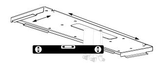
3 Install the radiator module on the support plate. Be careful not to trap the tubes when rotating the module.
